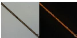
Optical (left) and POM (right) images of the C<sub>8</sub>-O-BTBT-OC<sub>8</sub>/F<sub>4</sub>TCNQ crystals
